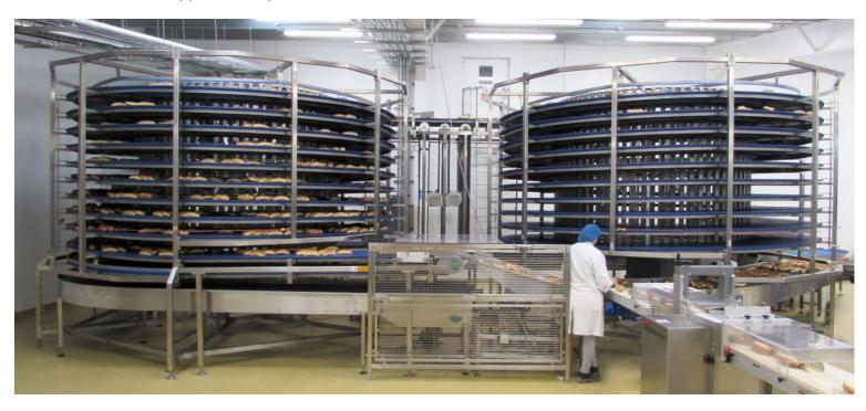
The total height of the system is 3340mm, the diameter of the spirals is 4526mm and the total length of the system is 10176mm.
