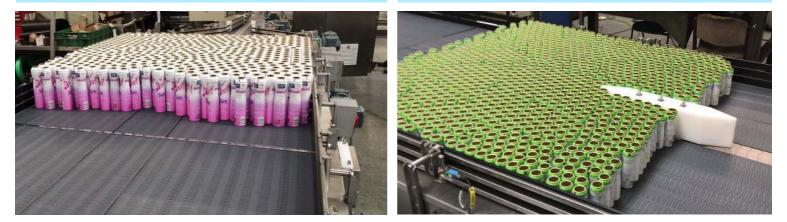
Unitech Engineering worked closely with our client to design and manufactured two bespoke de-palletiser tables. Our client requested from the start of the project that we adhere to their mechanical and electrical standards and specifications. This included us using their preferred suppliers for some of the components.
